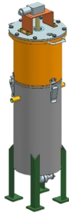
Figure 7 Detail 3D of generator hydrogen on demand
