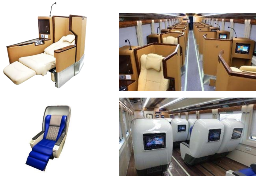
Figure 2 Design of the first and second generation of luxury sleeper passenger seats used in the questionnaire.
