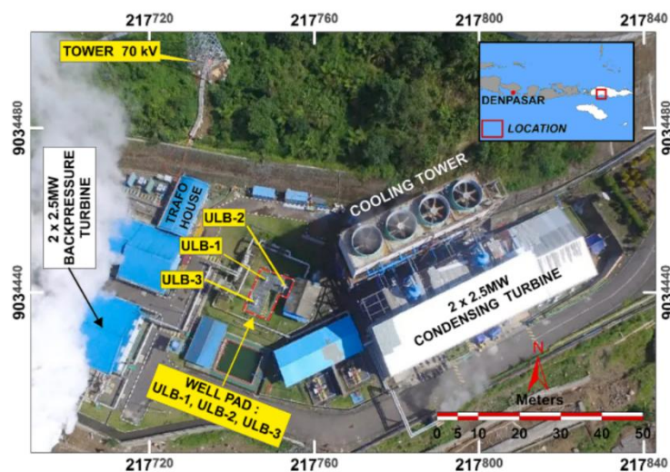
Figure 1 Ulumbu Geothermal Power Plants and a Well-Pad: ULB-1, ULB-2, ULB-3 [5].
