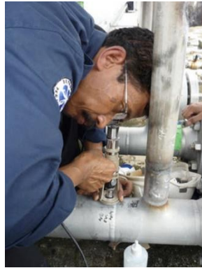
Figure 1 illustration of inspection using in-situ metallography kit [3]
