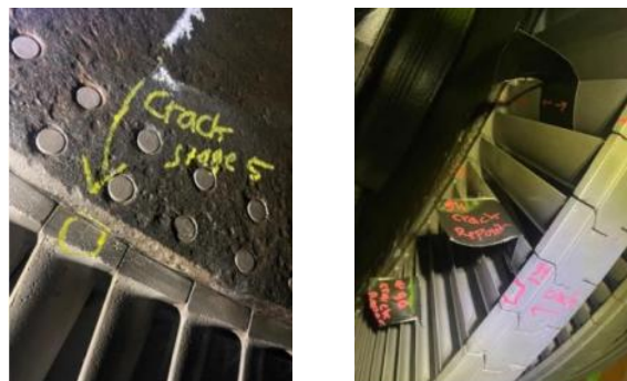
Figure 3 Crack presence on the shroud and root of the stage-5 turbine blade [4]
