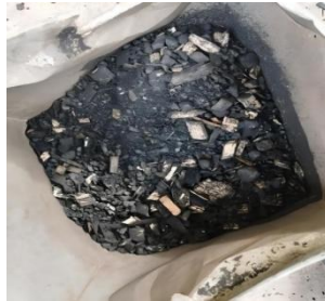
Figure 1. Fuel mixing Woodchips-Coal
