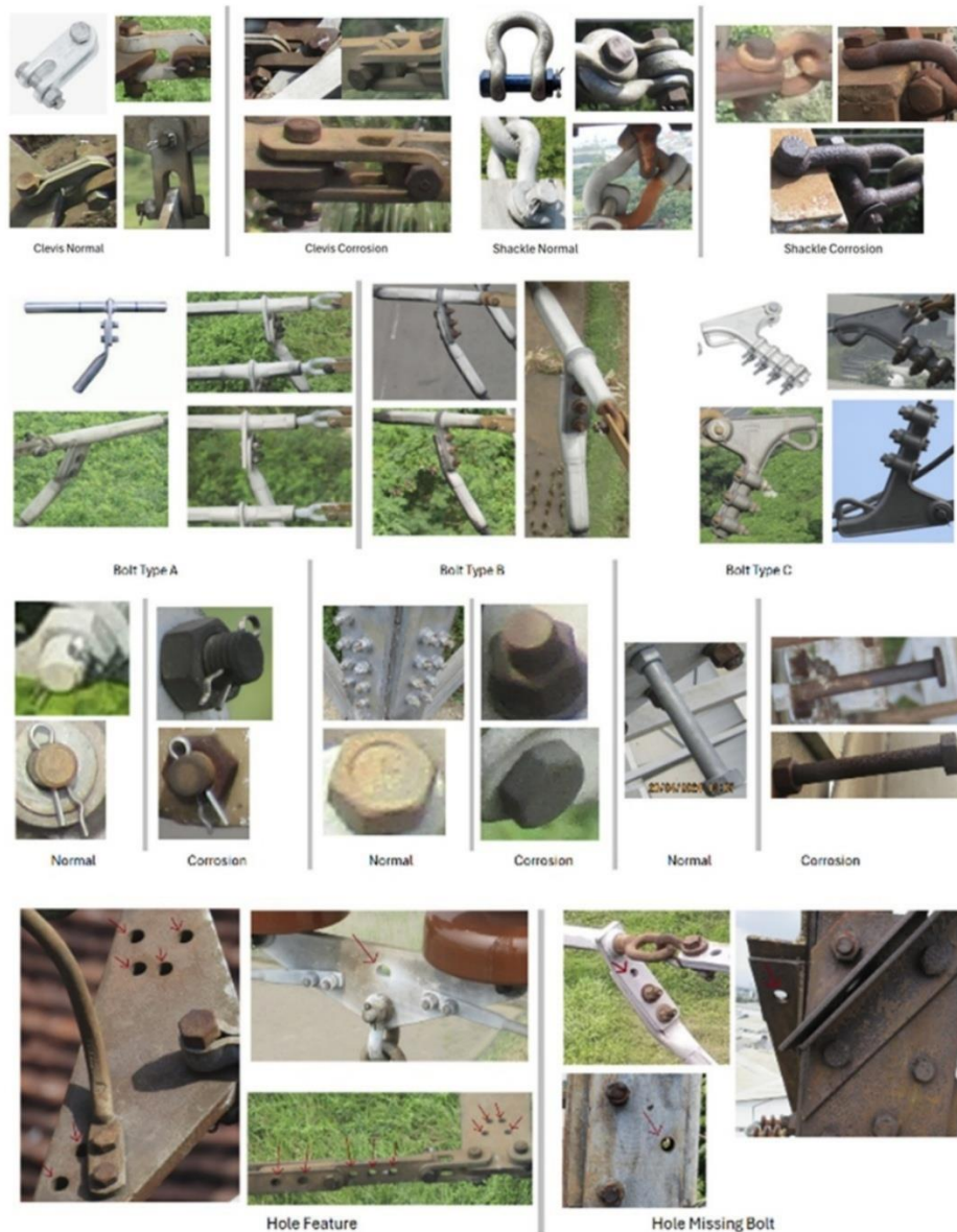
Figure 2 1 st Row: Clevis normal and corrosion (left) and Shackle normal and corrosion (right), 2 nd Row: Dead End normal and corrosion (left) and Tension Clamp (right), 3 rd Row: Bolt type A (left), type B (middle) and type C (right), 4 th Row: Hole Feature (left) and Hole because missing bolt (right)
