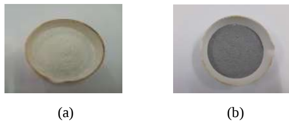
Figure 1 Duck Eggshell Powder (a) Before Calcination (b) After Calcination
