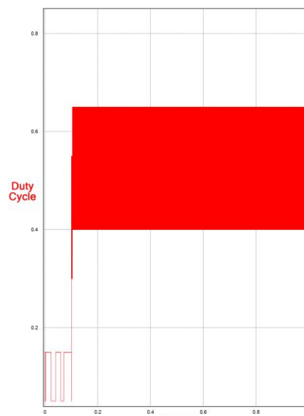
Figure 11. Duty Cycle of P&O Method
