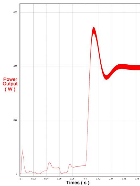
Figure 10. MPPT Power Graph with P&O Method
