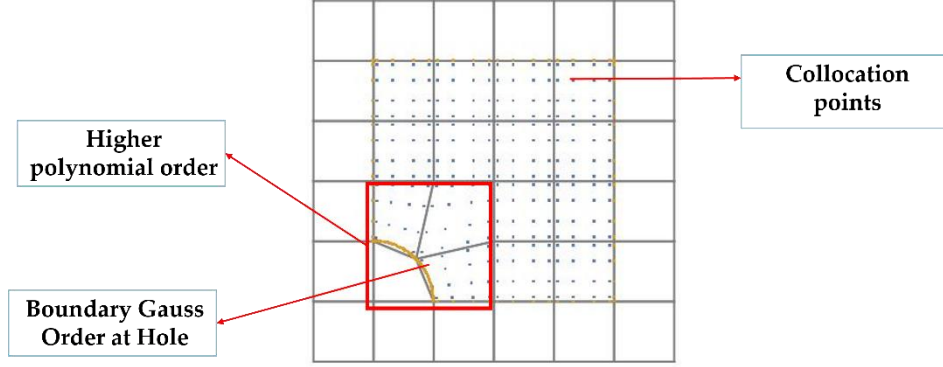
Figure 5 Local p-adaptivity implementation on plate with hole simulation using mollified collocation method
