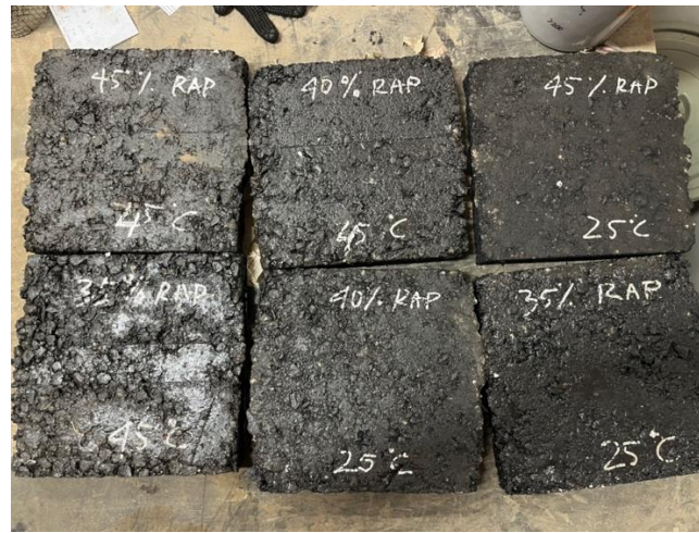
Figure 8 The Specimens Condition After Wheel Tracking Test
