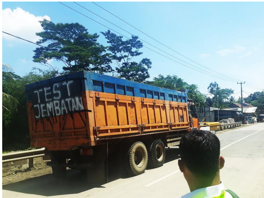
Figure 2 Pre-weighed truck for calibration
