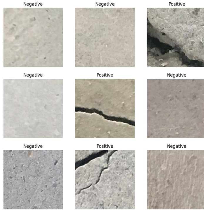
Figure 1 Some image examples from the training dataset for both the cracked and non-cracked concrete surfaces.
