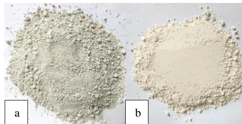
Figure 2. Soil texture of (a) bentonite and (b) \text{CaCO}_3
