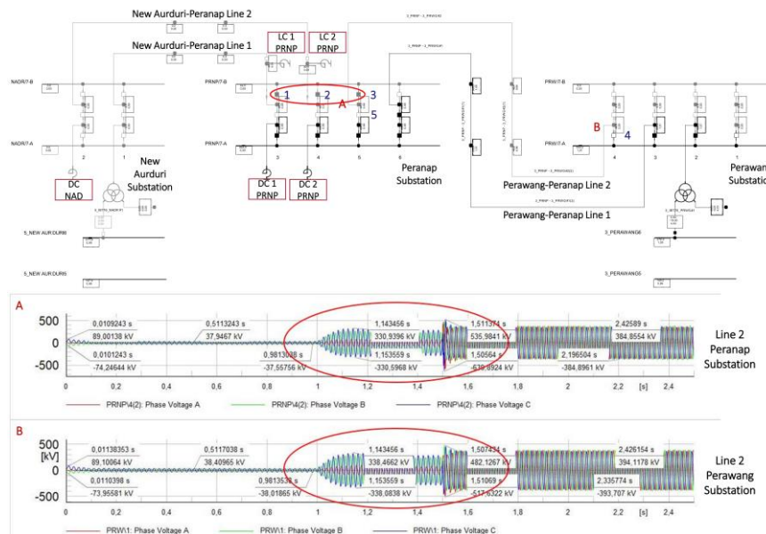
Figure 7 Resonance on the De-Energized Transmission Line (Line Connected Shunt Reactors)
